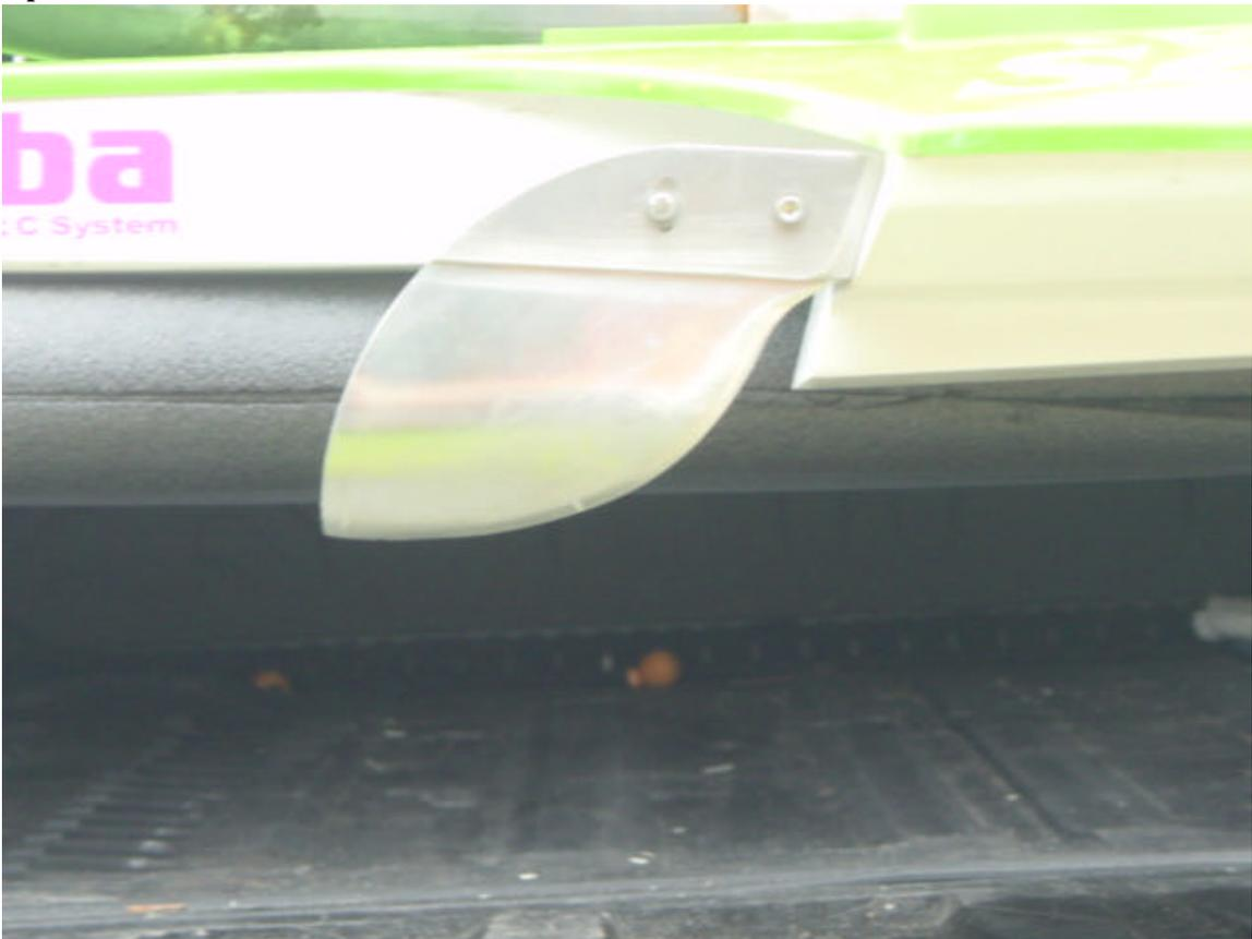
Turn Fin angle ( Roll Even with bottom of center section)
